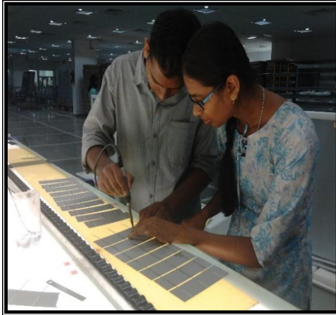
Putting solar cells in two rows
