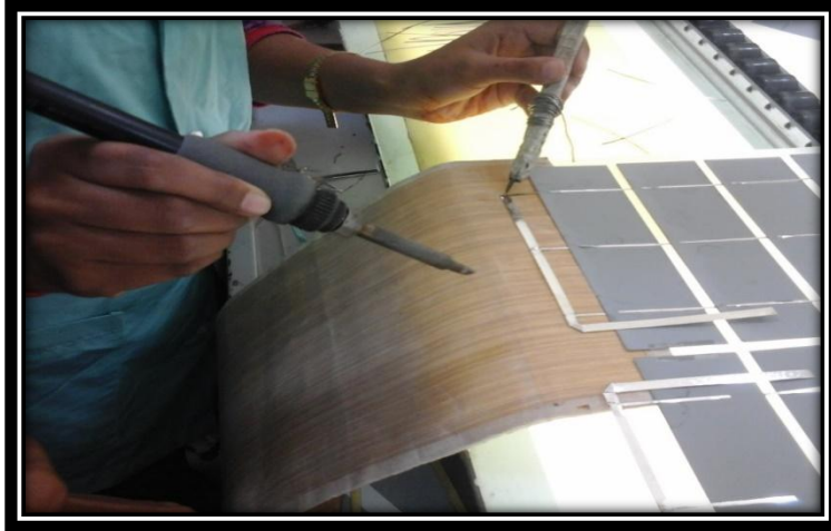
Connecting the tab wires of positive and negative terminal
