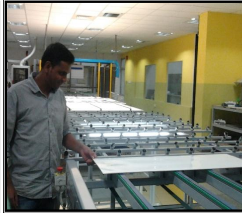
Tedlar sheet is being placed on the solar cells
