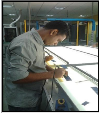
Tabbing of solar cells with interconnecting wires
